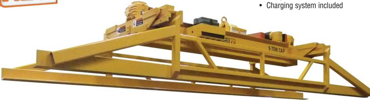
This Model 60BMS-5-96 will lift sheets up to 96" wide and uses full-time battery power to operate.
