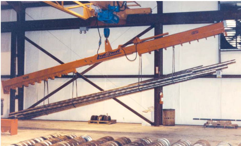
Special 4-point Posi-Leveler™ with load guides.
