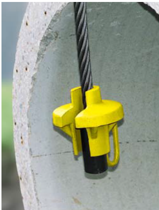
Drop pipe carrier lifting sling through hole in pipe. Align and insert “Tea Cup” pipe carrier into lifting sling.
