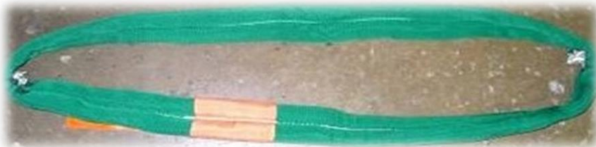
Sling #2 after ultimate load testing
