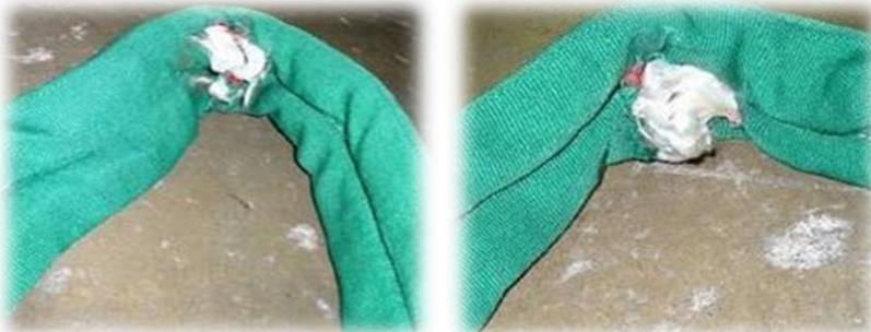
Close-up of each end of sling #2 after ultimate testing
