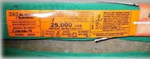
Close-up of tag on sling being tested
