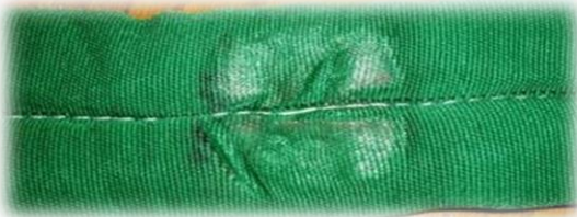
Photograph of the inside end of sling after cycle testing has been completed
