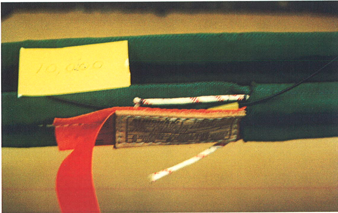
PHOTOGRAPH #2 TPXC 1000 SLING – STRAIGHT PULL @ 10,000#
